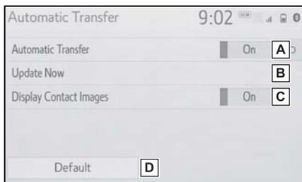
**A** Select to set automatic contact/history transfer on/off. When set to on, the phone’s contact data and history are automatically transferred.
