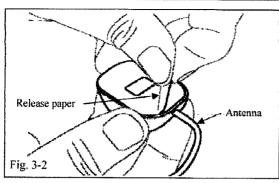
(3) Remove the release paper from the back of the antenna; then install the antenna onto the center of the ground plate.
