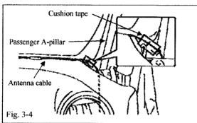
(5) Route the antenna cable toward the corner of the instrument panel near the Apillar. (Fig. 3-3, 3-4)
